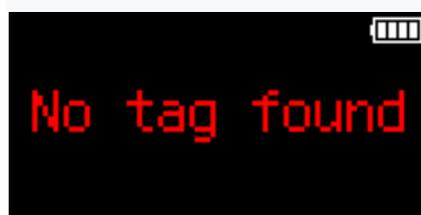
In this case, it is advisable to carry out new reading attempts, two to three times immediately by scanning the area more widely supposed implantation. Every new pressing the side button will restart the reading according to the process described previously.
