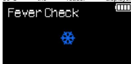
If the chip read is at a temperature above 42°C the reader displays:
